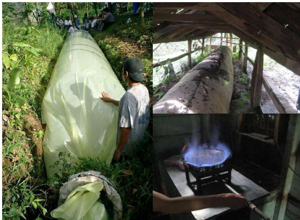
Figure 52. A simple anaerobic digester for pig manure and rests of food in the town of Bagaces (Costa Rica) to produce biogas that is used in kitchens.
