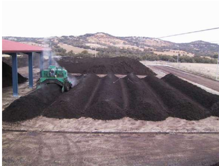
Figure 33. Composting windrows operated by a self-propelled turner.
