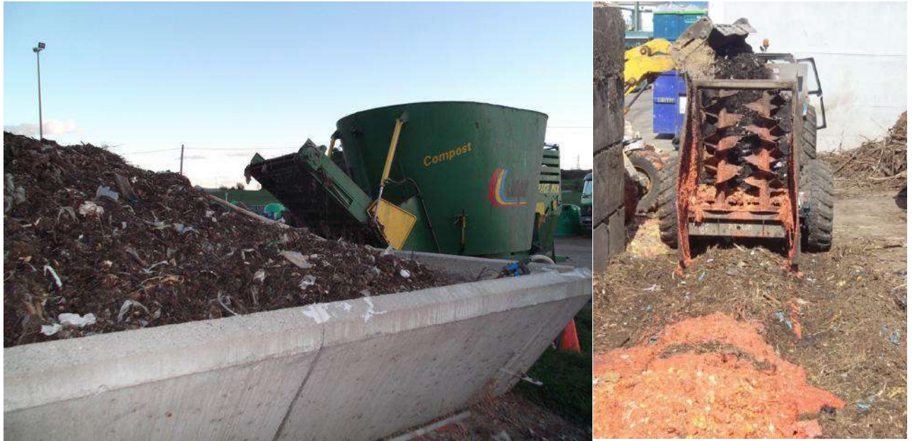
Figure 31. Other options of machinery for mixing and turning the materials. Left, feeder for cattle adapted to work like a mixer for biowaste and bulking; right, a trailer to spread manure used to mix the biowaste and the bulking material (it can also be used like turner machine).
