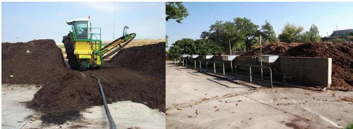
Figure 21. Left, type of lateral turner machine to realize the turnings of the composting plateaus. Right, a forced aerated system for static composting plateaus.
