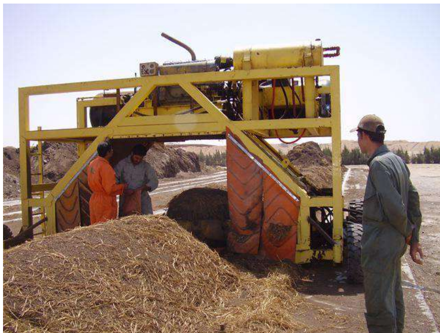
Figure 40. Self-propelled turner machine made locally in Egypt.
