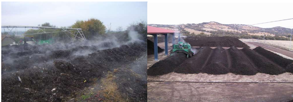
Figure 20. Left, static windrows with forced aeration by the Rutgers system. Right, dynamic windrows being turned by a turned machine.
