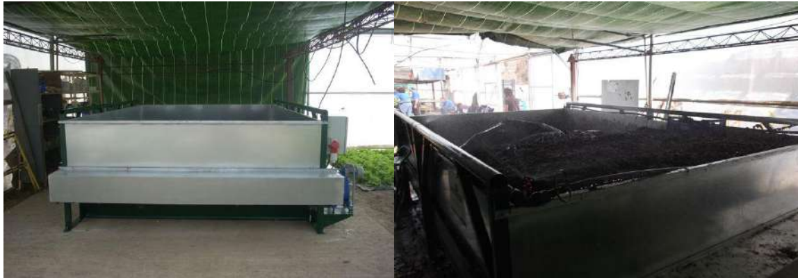
Figure 53.- An automatic vermicomposting system that allows a continuous feeding with organic waste by the upper side and the unload of the vermicompost by the bottom (Elkarkide, Navarra, Spain).
