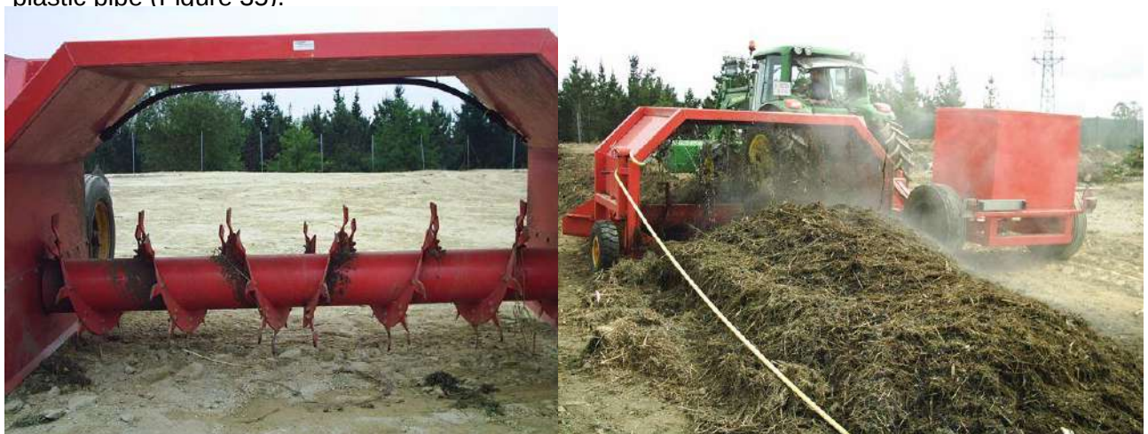
Figure 35. “Self-made” watering system for a towed turner. Left, it can be seen the perforated pipe linked to the rear part of the turner and with the length and form of the arch. Right, a hose is connected to the pipe during the turning and watering of the windrows.
