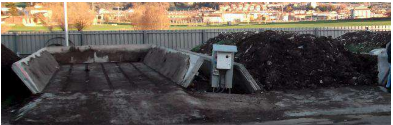
Figure 42. A force aerated composting system where it can be seen the ventilated area empty (left) and with the windrow in process (right).
