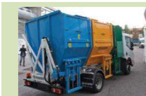
(a) Collection truck with three separate compartments inside, lateral load.
