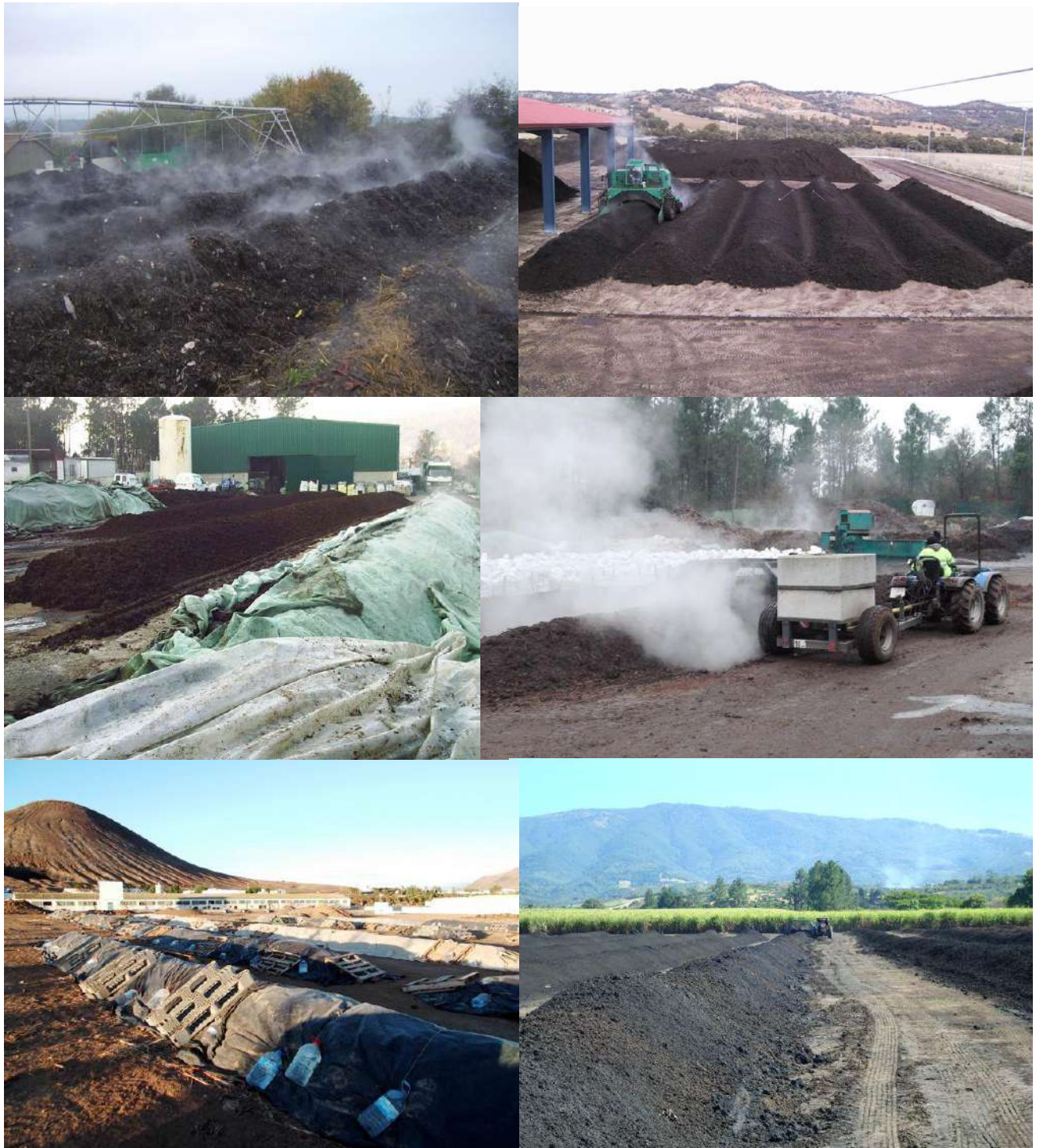
Figure 29. Examples of composting facilities with turned windrows.
