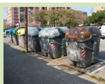
(b) Containers for Biowaste, Residual waste glass, paper-cardboard and lightweight packaging (side load collection) in Barcelona.
