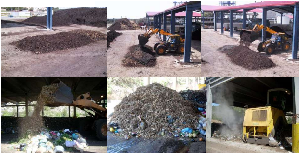
Figure 30. Sequence of formation of windrows with different biowastes. Upper line: left, layer of bulking material extended; center, unload of biowaste (swine manure) on the layer of bulking; right, covering the biowaste with another layer of bulking before the pass of the turner machine. Bottom line: left, covering household biowaste with bulking; center, aspect of the windrow before to be turned; right, turning the windrow to mix bulking and biowaste.
