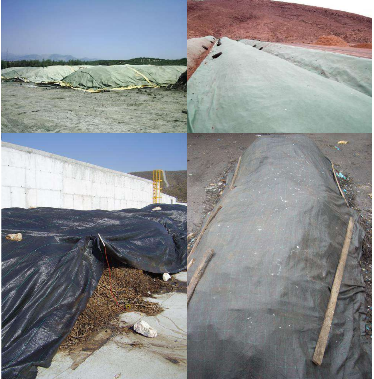
Figure 36. Different examples of covers or canvas for composting windrows. Upper left, Gore®Cover canvas; upper right, TopTex™ canvas; bottom line, anti-grass covers used in professional gardening.
