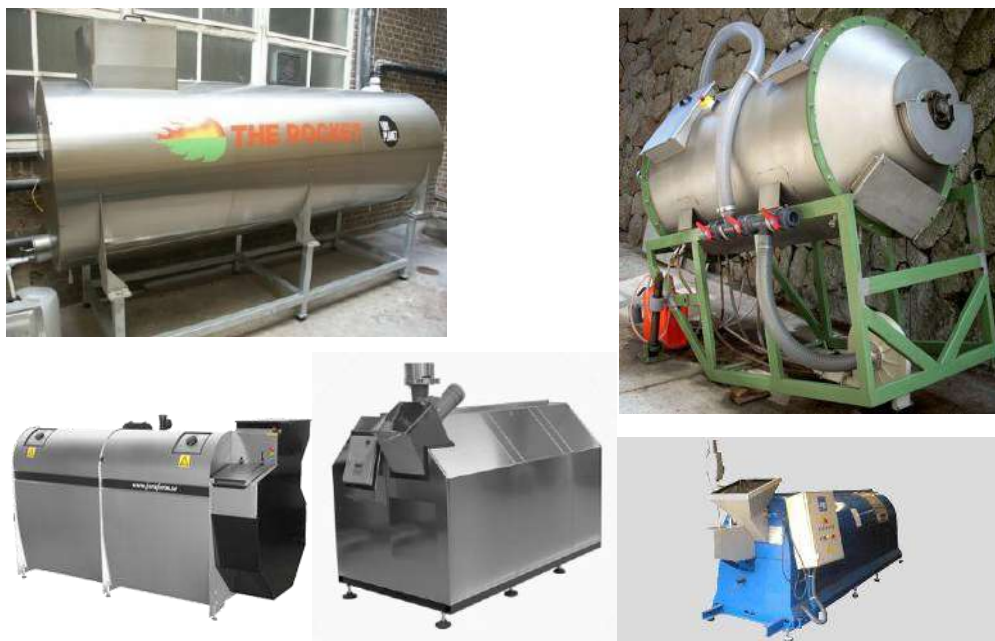
Figure 24. Different models of dynamic closed composters for household biowastes (Jora, Kollvick, BigHanna, Rocket, Campusteiro). All of them have a common structure (cylinder with agitation system). The differences are in the process control, the regulation of the retention time, the regulation of leachates, and the stability of the final product.
